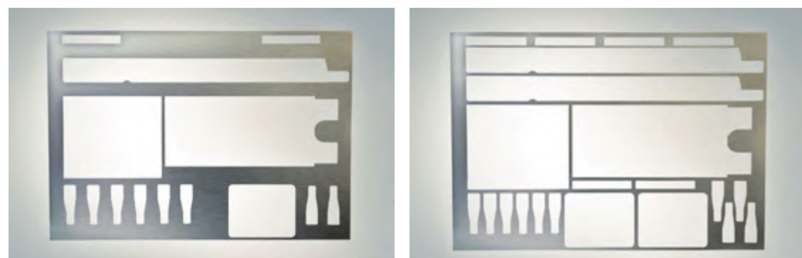
Figure 61: Left-over sheet metal following blanking of components in an unoptimized arrangement (top), and in an optimized arrangement (bottom), the latter creating much less left-over scrap
