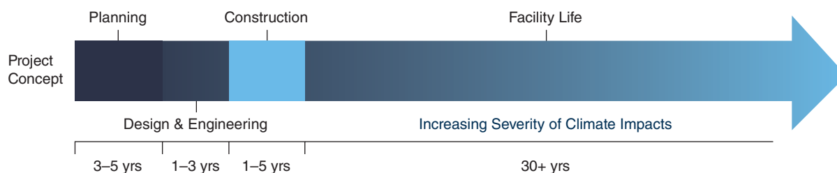
FIGURE 4 Climate Change in the Context of the Useful Life of Transport Infrastructure
