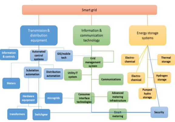
Figure IV Main pillars of the future "smart" grid
